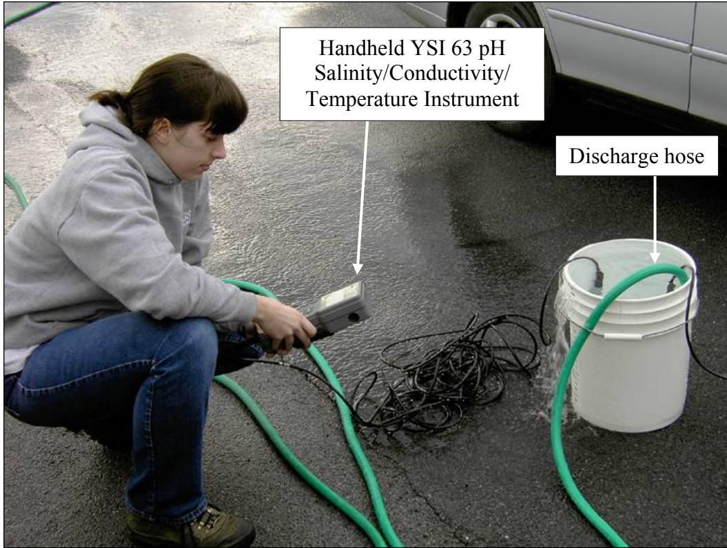
Figure 4-7. Water temperature, pH, and specific conductance of the ground water were measured during virus sampling.
