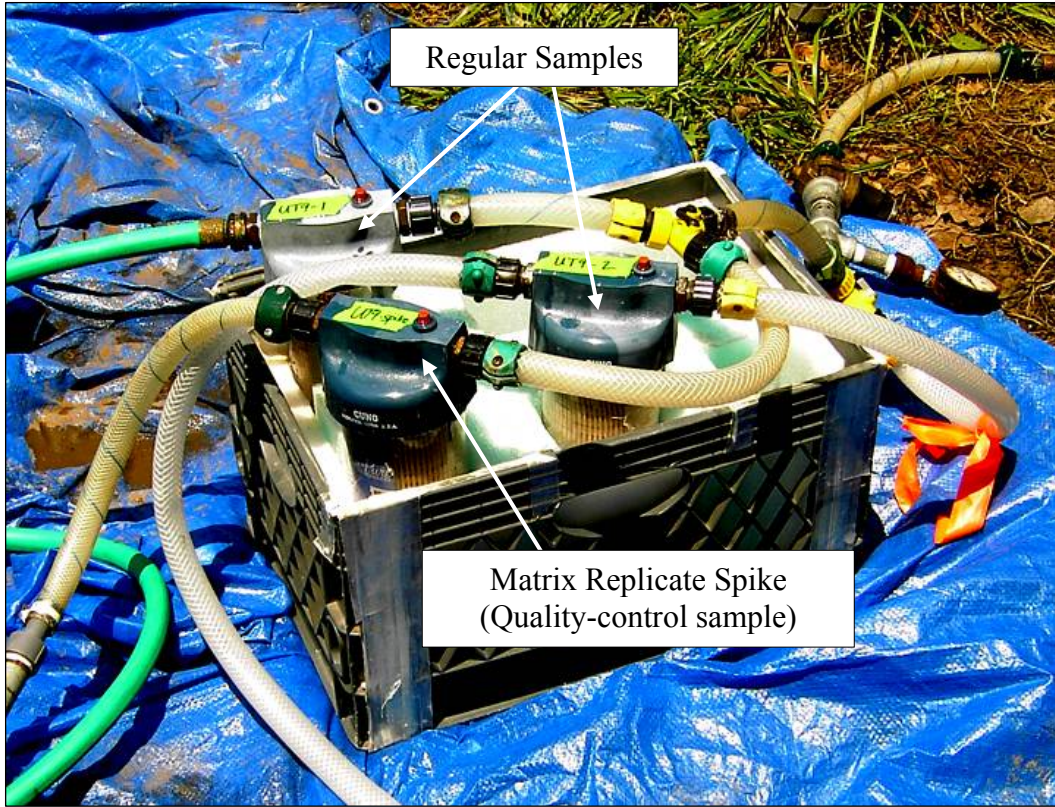
Figure 4-10. The flow into the virus sampling apparatus was split three ways to collect the matrix replicate spike and two regular samples.
