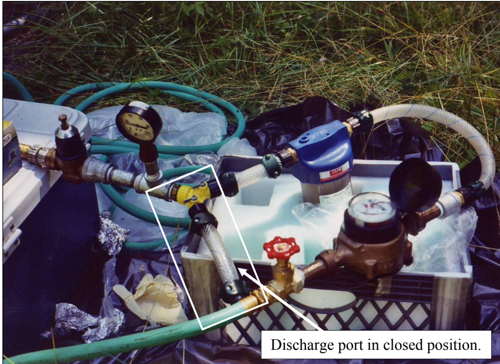
Figure 4-9. A short discharge port with an on-off valve was connected to the viral sampling apparatus.
