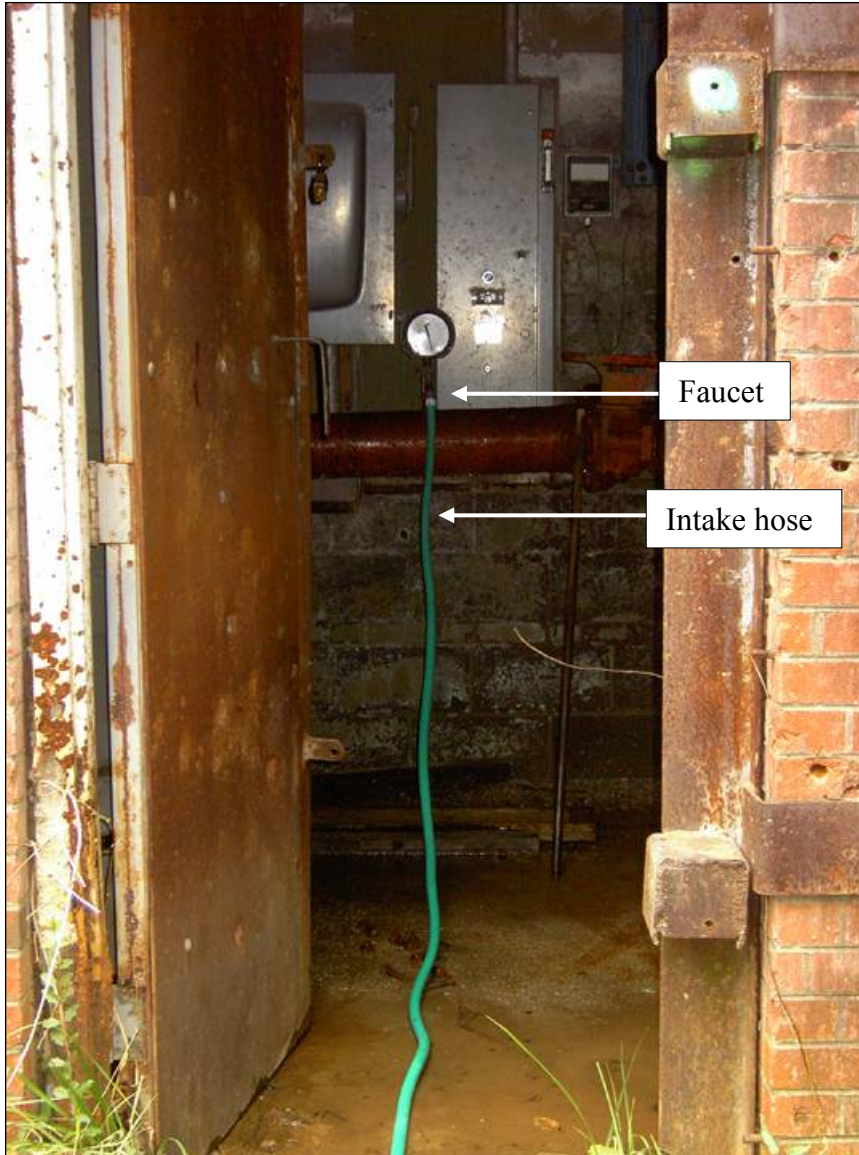
Figure 4-5. Intake hose for virus sampling apparatus connected to a faucet in a spring pump house.
