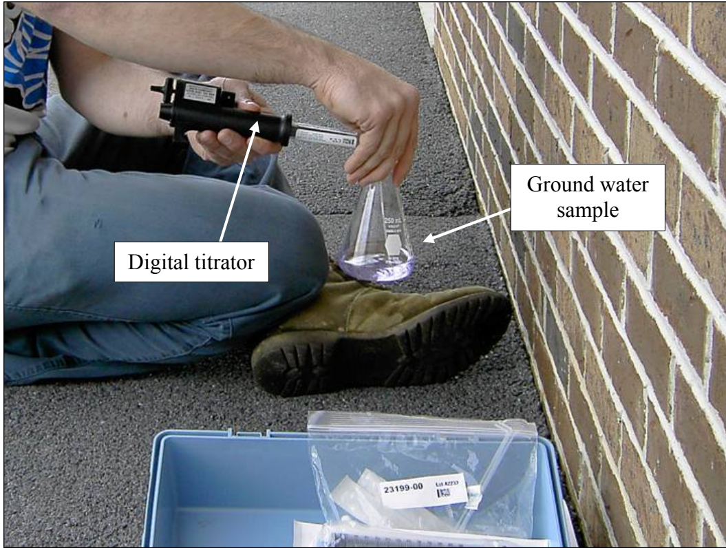
Figure 4-11. The alkalinity of a ground water sample is tested using a Hach titration-based test kit.
