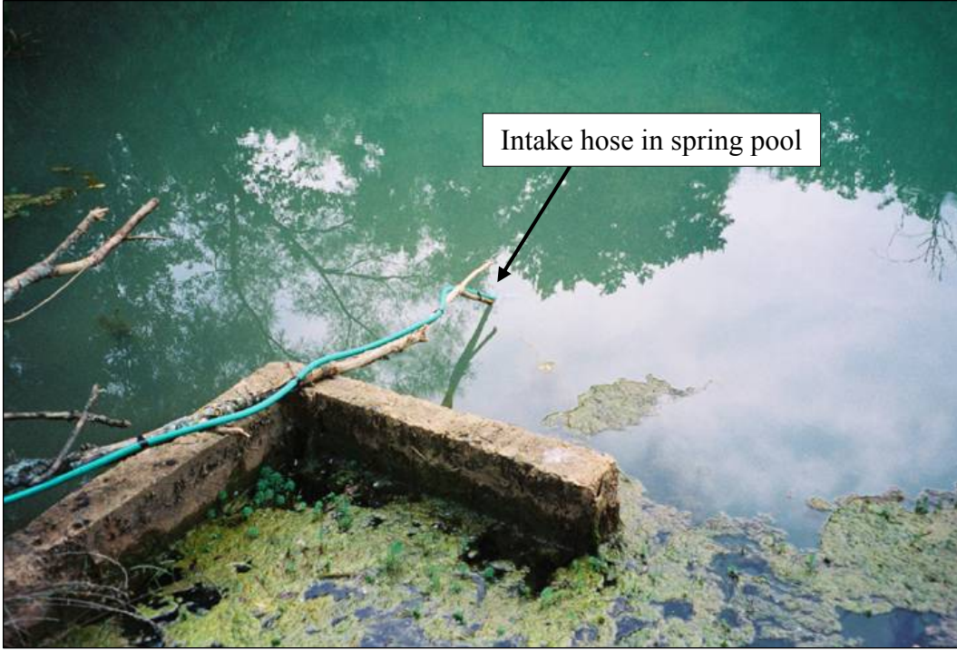
Figure 4-6. At site S-4, the intake hose for the virus sampling apparatus was put directly into the large spring pool.
